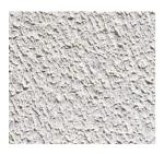
White Reflective helps to keep the liner cooler, resulting in fewer wrinkles. Fewer wrinkles mean the easier installation of cover soil and increasing the lifespan of the liner.
