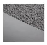
HDPE Series is a high-density polyethylene geomembrane that exceeds the requirements of the international and local specification standards for HDPE geomembrane liners. This series of geomembrane liners offers proven performance as a primary containment barrier in landfill applications.
